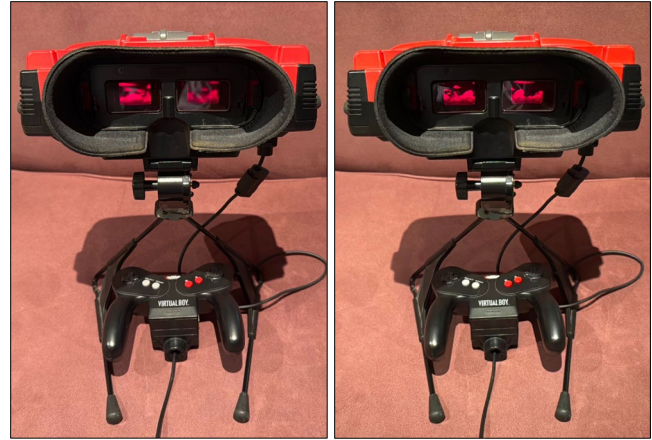
Figure 8. Stereo-pair of the original Nintendo Virtual Boy (cross-view format). Photo: Andrew Woods using an iPhone 15 Pro in Spatial Photo mode.
