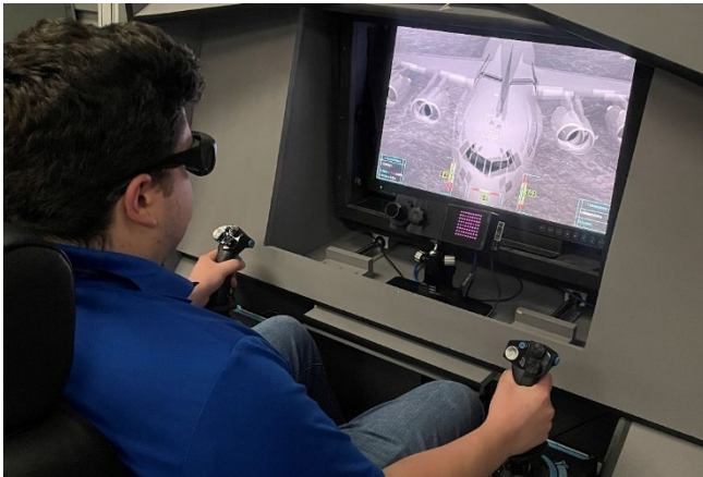
Figure 1. sRVS set-up with aircraft monitor, EyeLink eye tracker and Saitek flight control. Photo by OBVA Lab personnel.
