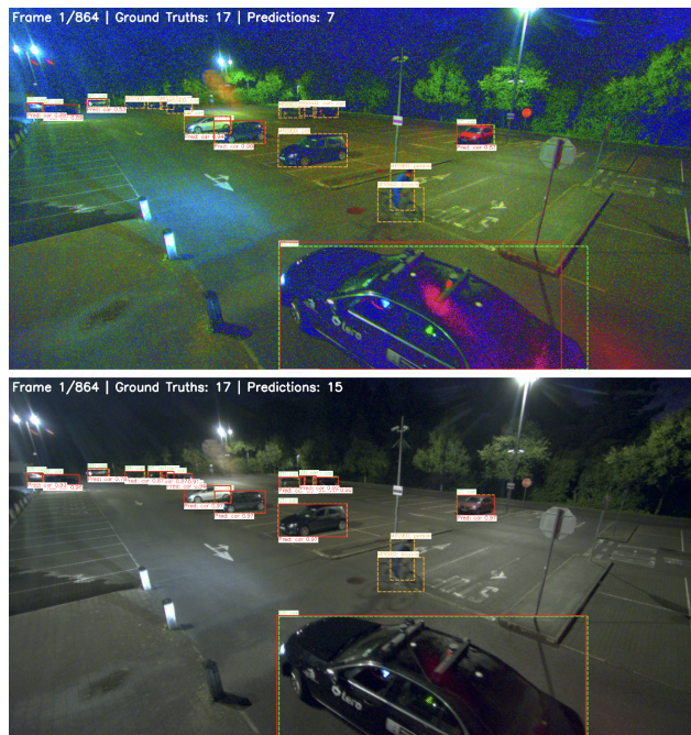
Figure 8. Detection results from YOLOv8m on the same scene processed with Saturation 2048 (top) and the default ISP (bottom). Green dashed: matched ground truth; orange dashed: missed ground truth; red solid: predictions.
