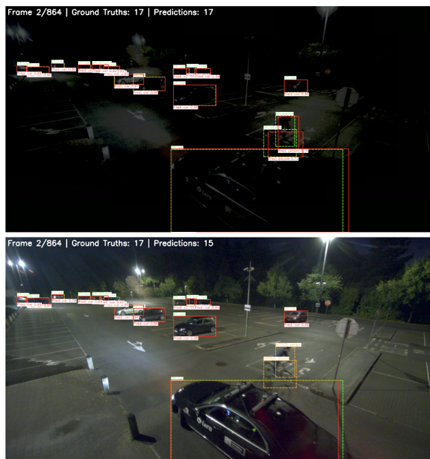
Figure 9. Detection results from YOLO26m on the same scene processed with Gain 8 (top) and the default ISP (bottom). Green dashed: matched ground truth; orange dashed: missed ground truth; red solid: predictions.
