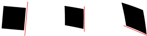
Figure 2. Distortion-induced transformation of edge orientation. (Left) Standard 5° slant providing uniform sub-pixel sampling. (Middle) Radial rotation toward 0° inducing phase collapse and a staircase ESF. (Right) An effectively 22° edge leading to oversampling rate shifts and orientation-dependent measurement bias.
