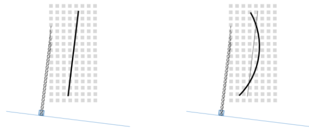
Figure 1. Comparison of spatial binning consistency and its impact on the Edge Spread Function (ESF). (Left) In a rectilinear system, linear projection correctly aggregates pixels with identical geometrical distances from the edge manifold, ensuring each sub-pixel bin captures a coherent phase. (Right) Radial distortion introduces a coordinate mismatch where the straight-line assumption fails to follow the curved manifold. Pixels at disparate true geometrical distances are erroneously aggregated into shared bins, artificially blurring the edge and degrades the reported SFR.
