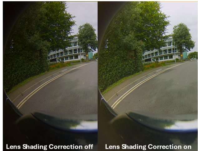
Figure 3. Illustration of lens shading correction for wide FoV cameras
