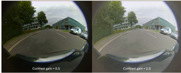
Figure 5. Durand tone mapping algorithm with 0.5 and 2.0 contrast gain
