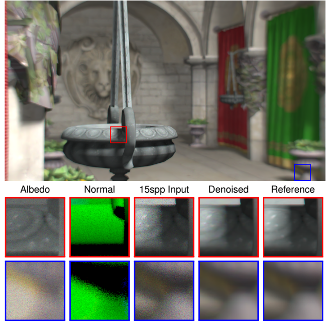
Figure 2: Sponza scene with 15 samples per pixel, denoised with OptiX Denoiser. Providing albedo and normal beside the RGB input lowers the denoiser error.
