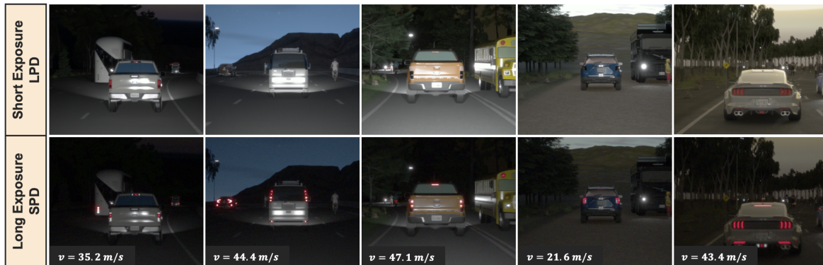
Figure 8. Dataset Diversity and Dual-Exposure Capture Analysis. Representative scenes from the ISET-LFM dataset illustrating the motion-flicker trade-off across varying environments. Top row (LPD): short-exposure (3–5 ms) and bottom row (SPD): long-exposure (11.11 ms), with ego-velocities ( v ) labeled for each scenario. These examples, generated via Option B, represent the separate radiance components provided in the dataset prior to HDR fusion.
