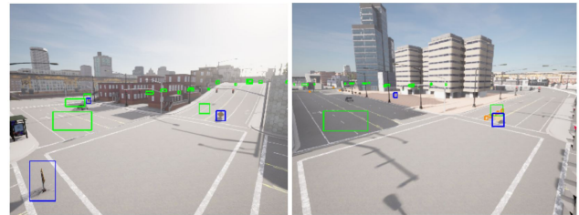
Figure 2: Test scenario with vehicle-RSU infrastructure in CARLA (Town05) showing false detections (green bounding boxes) and true detections (blue bounding boxes)
