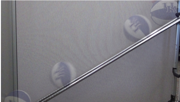
Figure 9: A virtual multiple exposure of a ball accelerating down a ramp.
