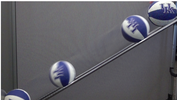
Figure 10: A motion study of a basketball accelerating down a ramp
