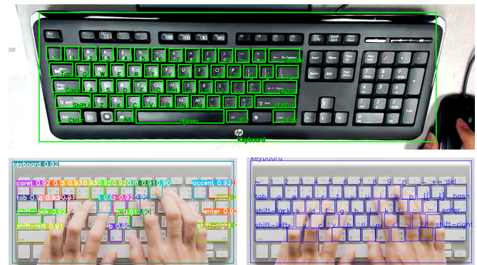
Figure 3. YOLO key detection on different types of keyboard images from MSU Typing Behavior Dataset [22] (top) and captured (bottom left). Example of key detection and hand-occluded key recovering (bottom right).
