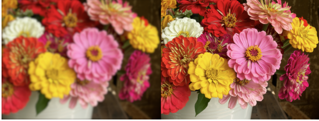
Figure 3. Example of two sharpness treatments corresponding to 15 and 0 JNDs of quality loss respectively, as defined by ISO20462[1].
