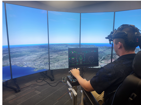
Figure 1: A photo over a participant's shoulder in the simulator. Five out-the-window (OTW) displays form a curve in front of the user, accompanied by a 27-inch monitor configured as a cockpit head-down display (HDD), and the AR HMD worn by the user.
