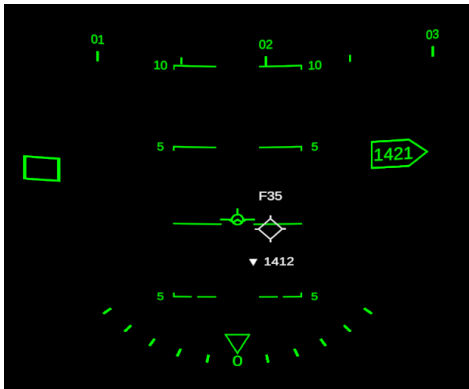
Figure 3: A screenshot of the symbology rendered to the OST AR HMD. The user's altitude appears to the right on the HMD, and a compass, pitch ladder, boresight, and bank indicator appear central on the HMD. In this example, the target plane symbol is drawn in white toward the center of the HMD. The user has already selected the plane and has designated it as an F35 within altitude range. Note that the black regions of the image will appear transparent to the user, such that only the green and white imagery is visible.
