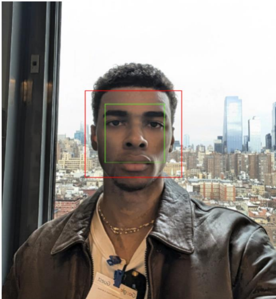
Figure 5. Face ROI by face detection (red rectangle), and modified face ROI passed to the post-ISP for face color evaluation
