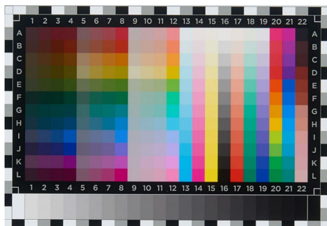
Figure 9 – IT8 Color reflection target for input scanner calibration
