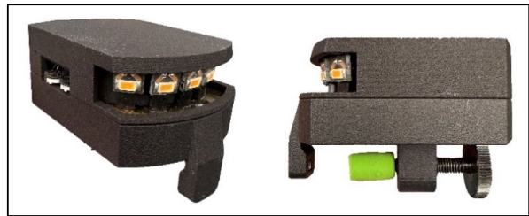
Figure 12. The 3D synchronizer for active 3D compatible OLED monitors developed by Peter Giokaris and discussed in his presentation. (Photo: Andrew Woods)
