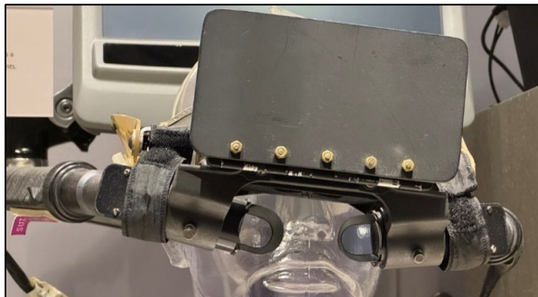
Figure 33. Closeup view of the "Sword of Damocles" head-mounted display showing what appear to be half-silvered mirrors at the view-pieces and a hinged panel which can presumably be lowered to block the view of the real-world. (Photo: Andrew Woods)
