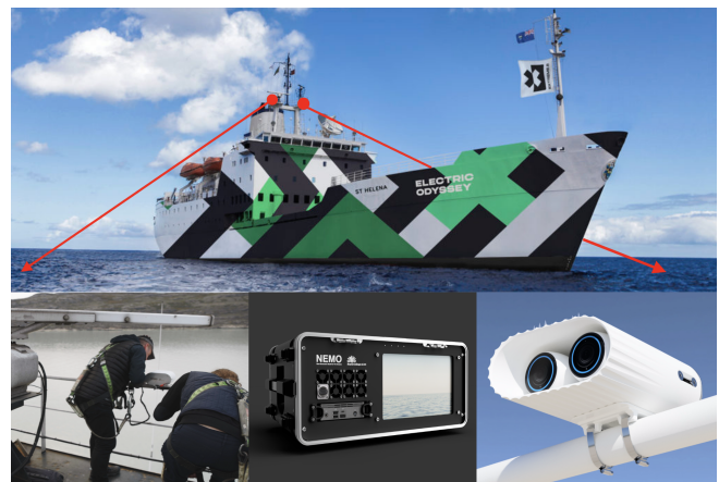
Figure 1. The St Helena ship showing camera location and angles (top), installation of cameras (bottom left), control unit and NVR's (bottom centre) and camera shroud (bottom right).
