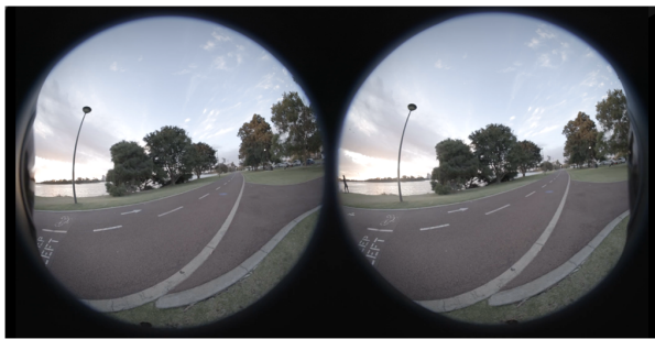
Figure 4: two side-by-side fish-eye 3D images captured by the Canon R5C camera fitted with the dual fish-eye lens.
