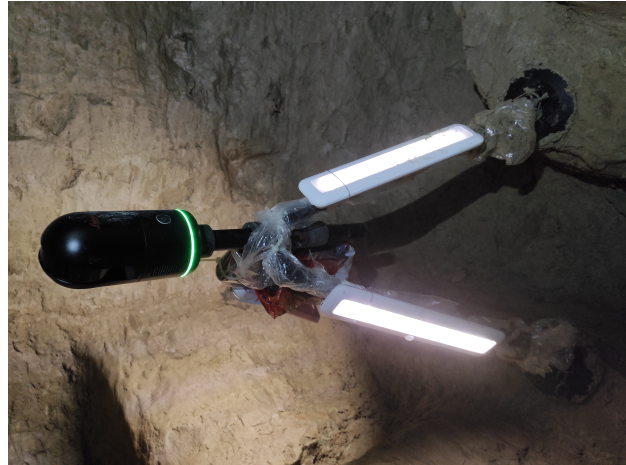
Figure 3. High-precision terrestrial LiDAR scanner: Leica BLK360 mounted on a tripod and equipped with additional lighting (left); Positioning the LiDAR above the crawlway to measure it as accurately as possible (right).
