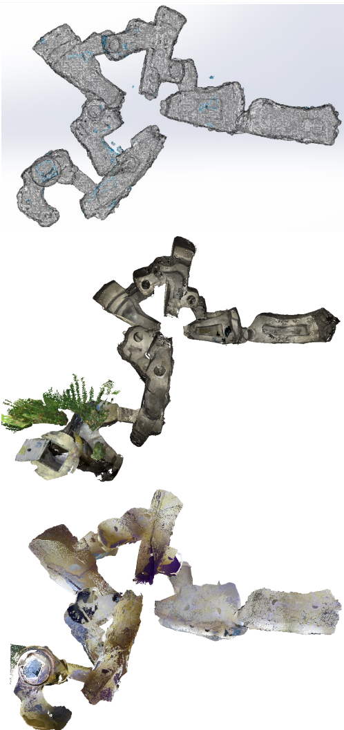
Figure 5. Comparison of the two measuring methods: (from top to bottom) speleologist survey original plan (photo: Erhard Fritsch, 1998); 3D survey using photogrammetry with Lenovo Phab2 Pro; 3D survey using with iPhone 15 Pro Max and top view with Leica BLK360.
