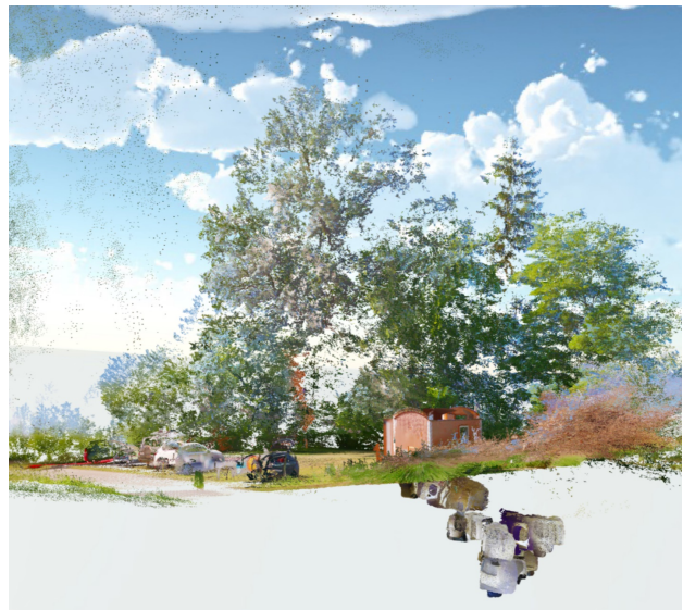
Figure 4. Above ground and underground surveying of Erdstall environment by LiDAR BLK360.
