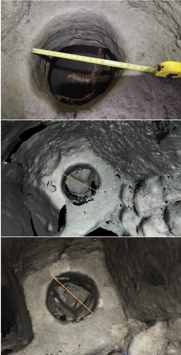
Figure 9. Comparison of the three measurement methods for vertical crawlway (diameter: 40.1 cm) between rooms 5 and 6. The measurement methods: 1. Speleological surveying; 2. Lenovo Phab2; 3. iPhone 15 Pro Max.
