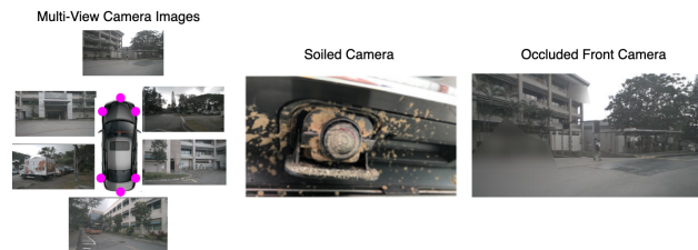
Figure 1. Left: Multi-view cameras and their mounting positions on the ego vehicle. Middle: Camera lens obstructed by mud, raindrops, dust, etc. Right: Occluded image
