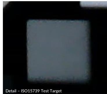
Figure 2 Detail of ISO15739 test target. The noise increases significantly close to the edge, showing that the flat gray area is processed differently
