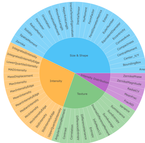
Figure 4: Overview of Feature Categories and Subtypes Extracted by PySpatial. The diagram illustrates the 247-dimensional feature space categorized into Size & Shape, Texture, Intensity, and Intensity Distribution, with representative subtypes shown in the outer ring.
