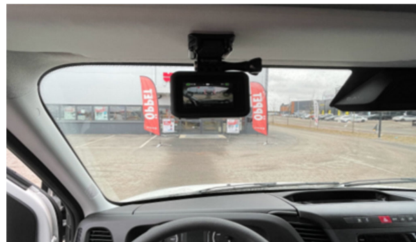
Figure 2: Mounting of interior camera for creating the forward view in experiments.
