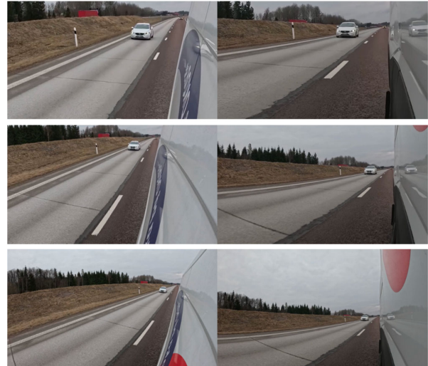
Figure 3: Same instance snapshots recorded with the two cameras at their respective camera height and FOV , the first column (left) for high camera, the second column (right) for conventional. Rows show the different FOV s. First row (top) 40, second (middle) 76, and third (bottom) 112 degrees.
