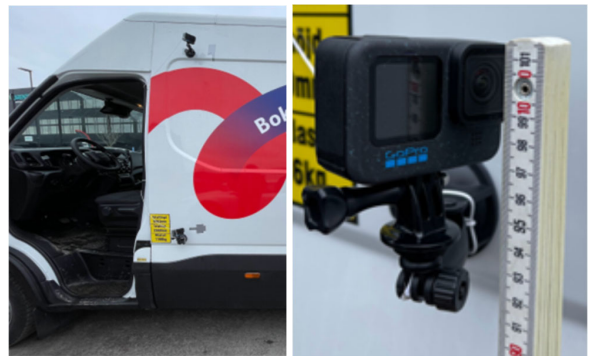
Figure 1: (left) Mounting of conventional (bottom) and high (top) camera heights. (right) Mounting for the conventional camera position, with the lens at a height of 1 meter from the ground.
