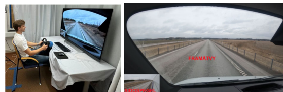
Figure 4: (left) Set up of the test room with the fixed positioning of the participant. (right) Screenshot of a simulated front view (Swedish: framåt) and side view mirror/camera (Swedish: sidospiegel) as presented in the experiments.
