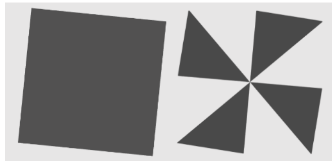
Figure 1. (left) ISO 12233:2017 slanted square. (right) ISO 12233:2023 four-cycle slanted star.
