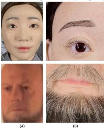
FIGURE 2. TWO ROIS WERE DEFINED ON EACH MANNEQUIN TO CAPTURE DIFFERENT DETAIL LEVELS (A) ROI FOR LOW-QUALITY CAMERAS AND (B) ROI FOR HIGH-END CAMERAS FOR FINE DETAIL EVALUATION.
