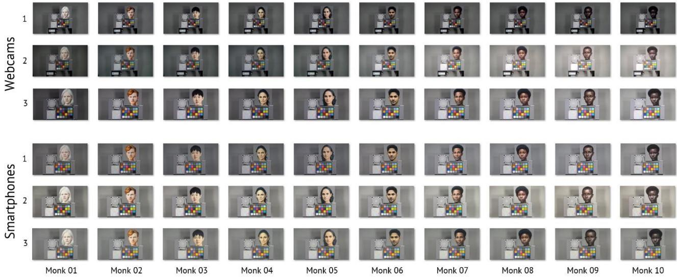
**Figure 9.** Frames extracted from video clips captured by three webcams and three smartphones under 6200K 250 lux illumination. Note the gradual increase in overall brightness as the skin tone in the scene becomes darker, despite being captured under identical lighting conditions.
