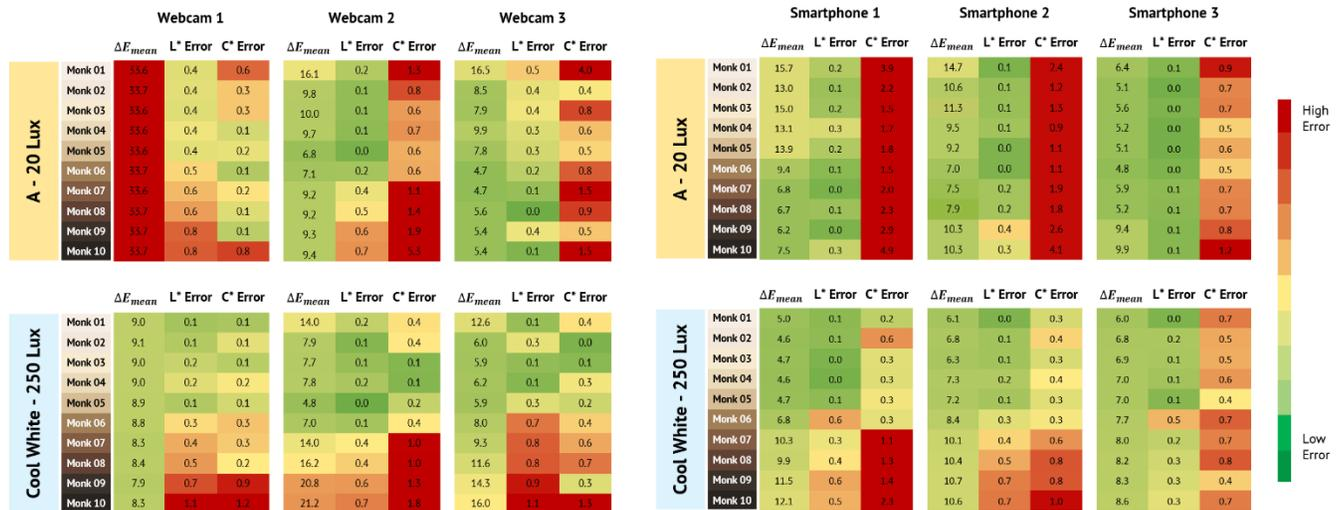
**Figure 10.** Three metrics of interest—average  $\Delta E_{2000}$ ,  $L^*$  error, and  $C^*$  error—calculated across devices, skin tones, and select lighting conditions. Values are color-coded according to deviation from target values.
