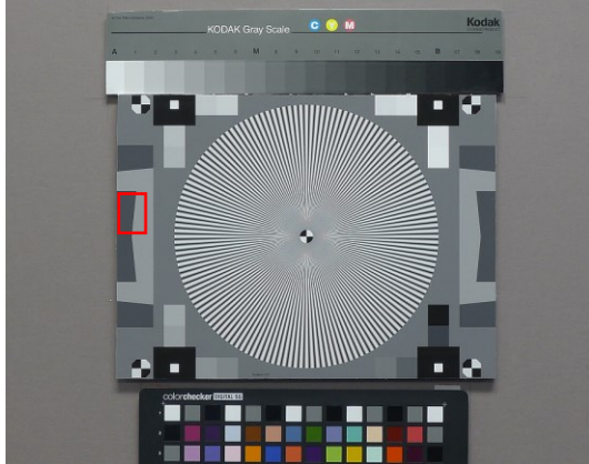
Figure 11. Typical image (cropped) including Siemens star and slanted-edges to the left and right of the star.
