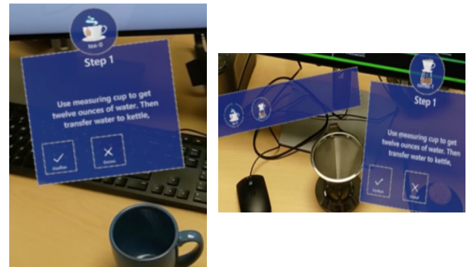
Figure 6 Once a recipe is selected, the instructions automatically anchor to a focal object for the recipe in the user’s view (e.g., mug). When multiple tasks are in progress, the task bar shows an icon for each task and the dialog for the non-focal task can be compressed to just its icon. The background color of the task icon shows its status.
