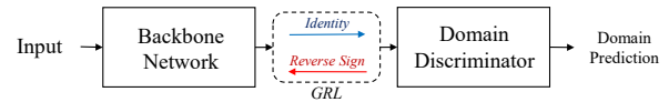
Figure 2. The gradient reversal layer (GRL) of the proposed model. The GRL layer is inserted between the backbone network and the discriminator network. During backpropagation, we multiply the gradient from the discriminator by -1 to reverse the sign of the gradient. In this way, the backbone network is trained to maximize the loss of the domain loss, which results in domain invariant feature extraction of the backbone network, and improved generalization capability.
