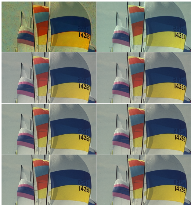
Figure 9. Quantized network output results on Kodak image number 9: (a) - 6 bit; (b) - 7 bit; (c) - 8 bit; (d) - 9 bit; (e) - 10 bit; (f) - 11 bit; (g) - 16 bit; (h) - float.
