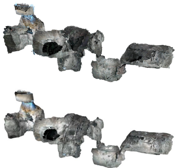
Figure 5. Map-Generation as 3D point cloud (top) and 3D mesh (bottom).
