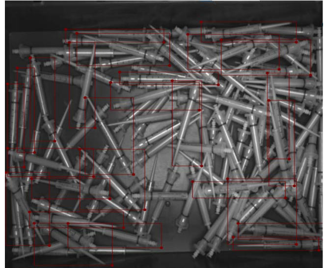
Figure 7. Camera image of a random arrangement of syringes in a box. The detections from an AI-based object detector, trained solely on synthetic data, are depicted with red bounding boxes.
