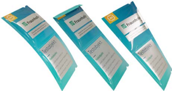
Figure 4. The original object model is bent (left and middle) and twisted (right).
