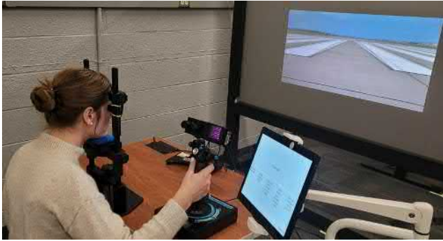
Figure 1. Apparatus showing chin rest, eye tracker, RVS screen, and survey tablet.
