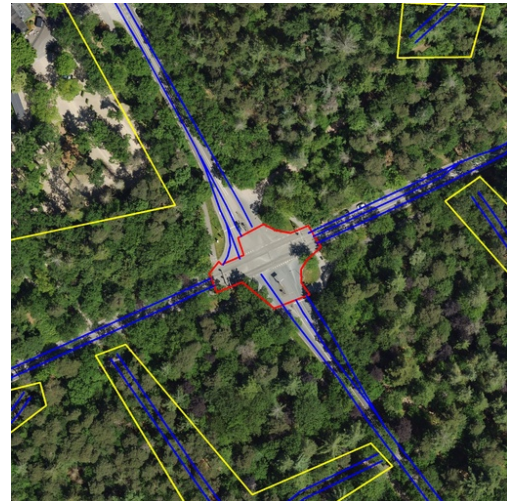
Figure 1. Example of annotated drive lines (blue), the conflict area (red) and ignore zones (yellow).
