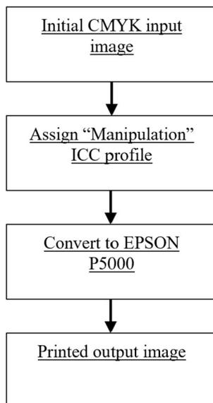
Figure 5. Flowchart to illustrate print production process.
