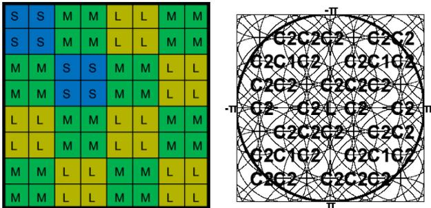
Figure 9: Double binnable LMS CFA (left), and its spectrum (right).
