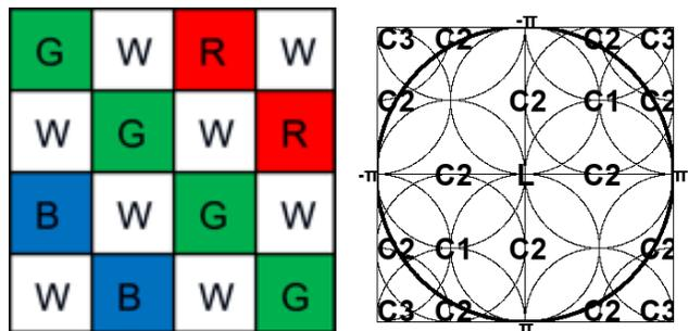
Figure 4: RGBW-Kodak CFA (left), and its spectrum (right).
