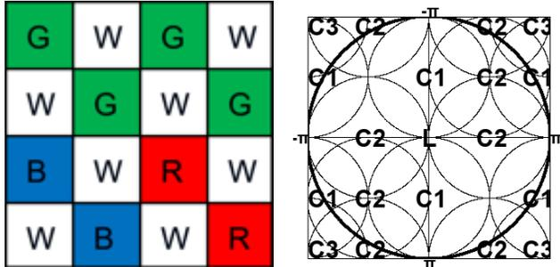
Figure 5: RGBW-IA CFA (left), and its spectrum (right).
