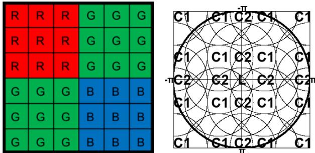
Figure 1: Nona Bayer CFA (left), and its spectrum (right).
