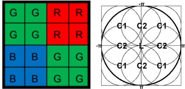
Figure 3: Quad Bayer CFA (left), and its spectrum (right).
