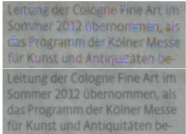
Figure 10: Newspaper (top), captured by a smartphone Quad Bayer CFA, converted to Bayer by the on-sensor remosaicker and then demosaicked by the state of the art algorithm of [12]. The same newspaper (bottom) captured by an equivalent sensor with the RGBW CFA and demosaicked with the algorithm of [8]. Note the poor legibility and severe artifacting in the Quad Bayer image.
