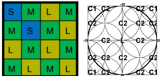
Figure 8: Single binnable LMS CFA (left), and its spectrum (right).
