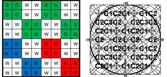
Figure 7: Quad-RGBW CFA (left), and its spectrum (right).
