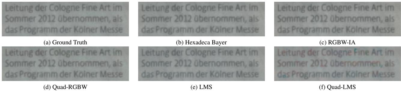
Figure 11: Simulated mosaicking of the Newsprint image with the Hexadeca Bayer and proposed CFAs followed by demosaicking with the algorithm of [8].
