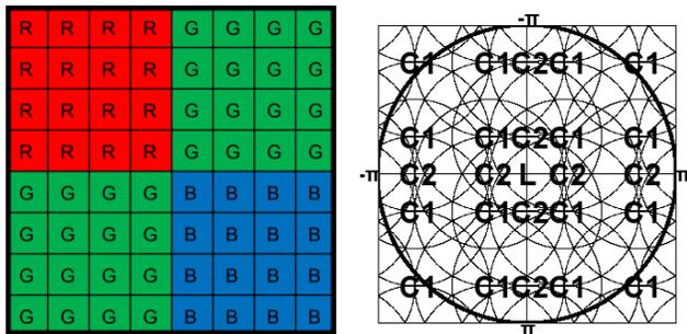
Figure 2: Hexadeca Bayer CFA (left), and its spectrum (right).
