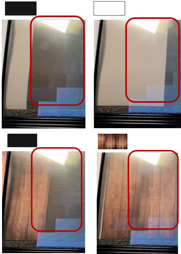
Figure 1. Visibility degradation according to the background brightness.
