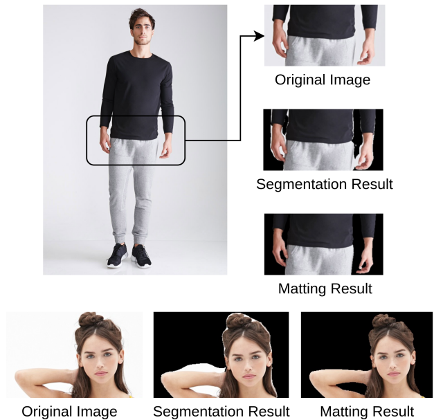
Figure 2. Comparing the segmentation and matting results. The matting method is better at accurately identifying the contour of the object compared to the segmentation method.
