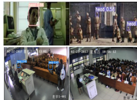
Fig. 3: Head detection results using Casablanca dataset for training yolov5 and testing the (a) Casablanca (b) Hollywood and (c) Scuthead dataset
