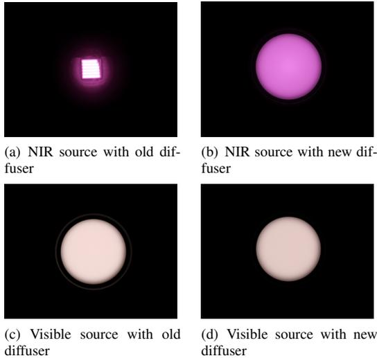
Figure 8. Diffusers on the visible and NIR sources
