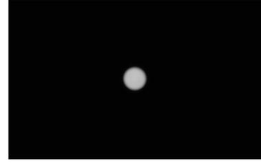
Figure 5. Uniform non-saturated gray level patch with  $x_0$ ,  $t_0$  and  $L_0$  the luminance of the source with the diffuser in front.
