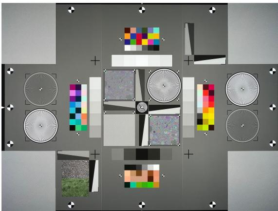
Figure 9. Target used for wide module evaluation.
