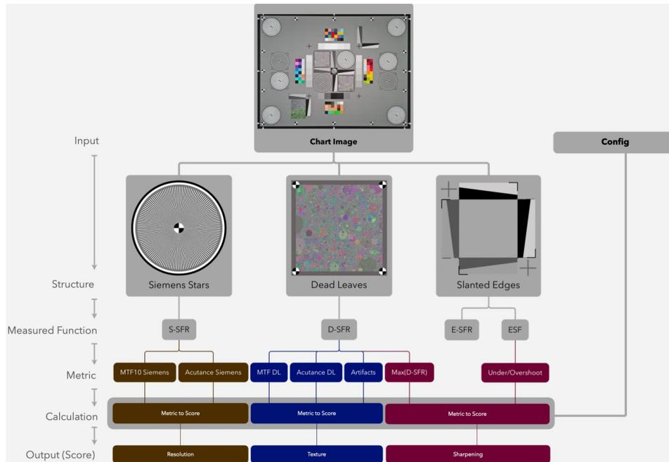
**Figure 11.** Different metrics form a group, these contribute to the total score depending on the weight per metric and per group. All measurements are performed per light condition.
