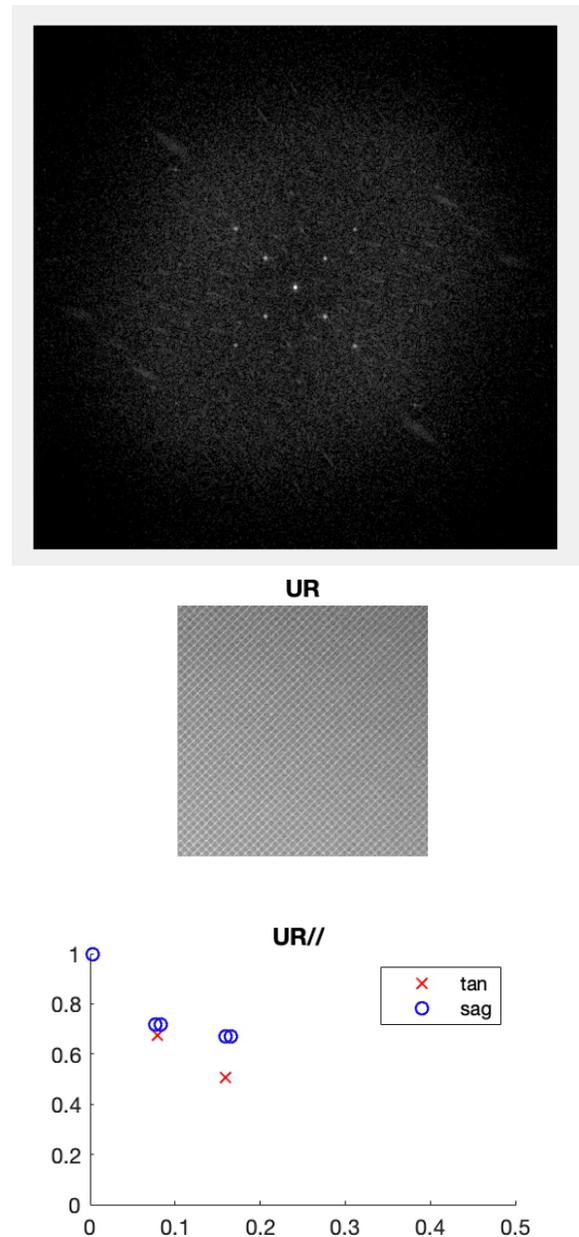
**Figure 10.** Top: Discrete spatial frequencies in the power spectrum of the image, showing the pattern. Down: Sample SFR obtained for one ROI (UR = Upper Right)
