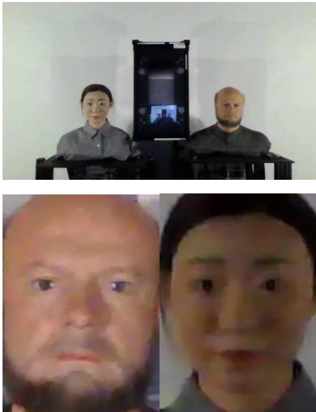
Figure 5. Example of Low-Quality Video Conference samples. From the complete setup (upper image) two Regions of Interest (ROI) are extracted, one for each mannequin.
