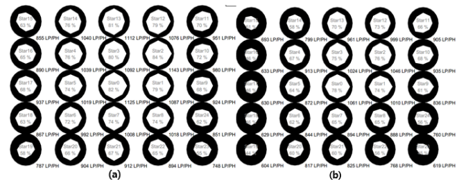
Figure 7. Resolution 20 Lux, (a) Conventional RGB Sensor Noise Reduction intensity level 5, (b) Nano Prism Sensor
