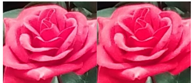
Figure 13. Maze Noise, Rose, Indoor (a) Conventional RGB Sensor (b) Nano Prism Sensor
