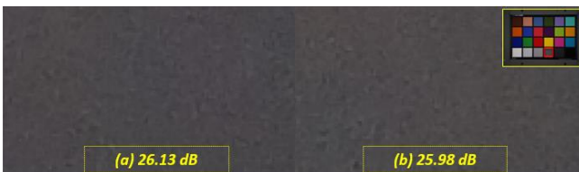
Figure 6. SNR 20 Lux, (a) Conventional RGB Sensor Noise Reduction intensity Level 5 (b) Nano Prism Sensor
