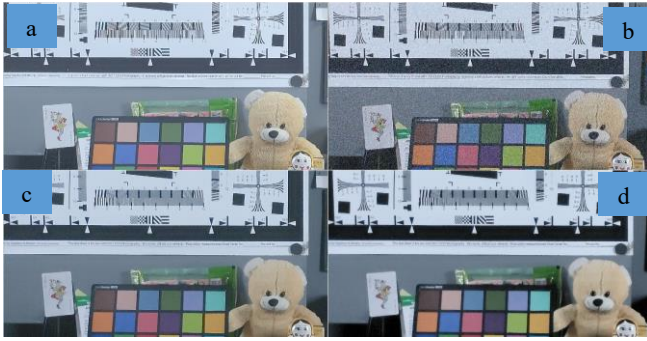
Figure 8: Subjective comparison of noise reduction and sharpness tuning done with different ISP parameters for Qualcomm ISP. a) 1000 lux reference image b) 10 Lux image tuned with default parameters c) 10 Lux manually tuned image d) 10 Lux image with optimized parameters (proposed approach)
