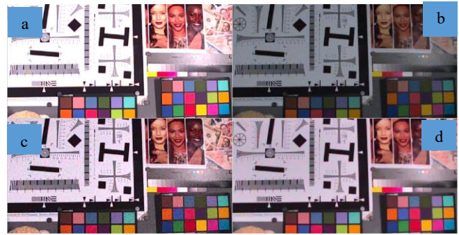
Figure 12: Subjective comparison of noise reduction and sharpness tuning done with different ISP parameters with TI ISP and 2MP sensor. a) 1000 lux reference image b) 10 Lux image tuned with default parameters c) 10 Lux manually tuned image d) 10 Lux image with optimized parameters (proposed approach)
