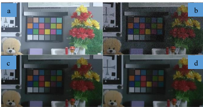
Figure 10 Subjective comparison of noise reduction and sharpness tuning done with different ISP parameters for Qualcomm ISP. a) 1000 lux reference image b) 1 Lux image tuned with default parameters c) 1 Lux manually tuned image d) 1 Lux image with optimized parameters (proposed approach)
