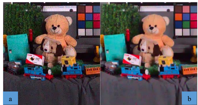
Figure 13 Subjective comparison of noise reduction and sharpness tuning done with different ISP parameters for 1Lux image with TI ISP and 2MP sensor a) Manually tuned image b) Image with optimized parameters (proposed approach).
