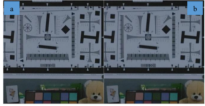
Figure 11 Subjective comparison of noise reduction and sharpness tuning done with different ISP parameters for 100Lux image with Qualcomm ISP. a) Manually tuned image b) Image with optimized parameters (proposed approach).
