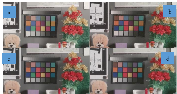
Figure 6 Subjective comparison of noise reduction and sharpness tuning done with different ISP parameters for Qualcomm ISP. a) High lux reference image b) Low Lux image tuned with default parameters c) Low Lux manually tuned image d) Low Lux image with optimized parameters (proposed approach)
