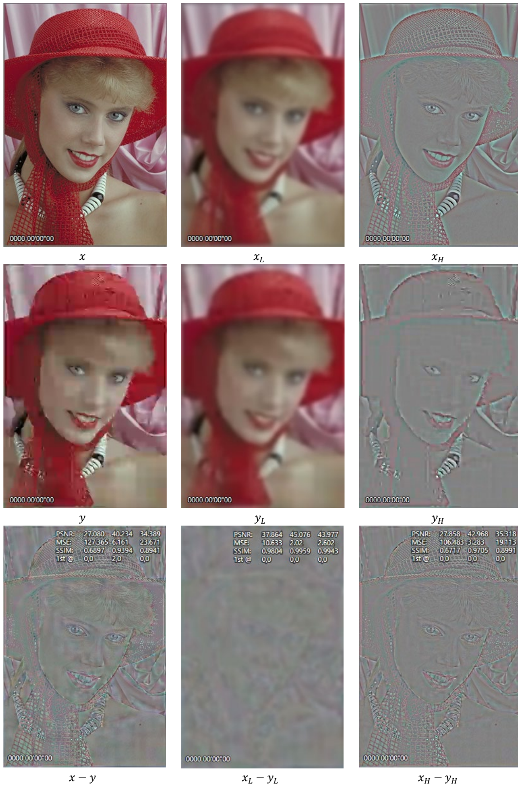
Figure 2. Visual illustration of steps in the proposed model for computation of SSIM. The top row shows an input image x and its low-pass x_L and high-pass x_H = x - x_L versions. The middle row shows the second input image y , and its low-pass y_L and high-pass y_H = y - y_L versions. This image is an encoded and decoded version of x , with significant distortions introduced by the codec. The bottom row shows the differences between the original images, as well as their filtered versions. Low-pass emphasizes changes in overall shapes, while high-pass emphasizes changes in textures, contours, and other fine features.
