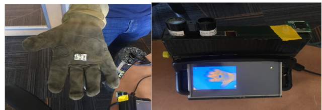
Figure 7. Thermal Reflectors for the Glove (left) and Thermal Imaging.
