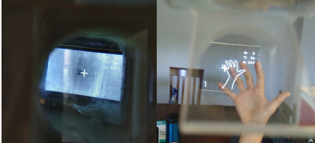
Figure 2. The overlaid thermal image (left) and contour (right) on the head-up display in the helmet.
