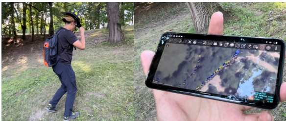
Figure 9. The firefighter walks in the field to take the ground temperature (left) and the cellphone maps the ground temperature data and transmits it to the command center (right).
