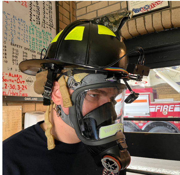
Figure 1. The thermal imaging and telemetry helmet for firefighters.
