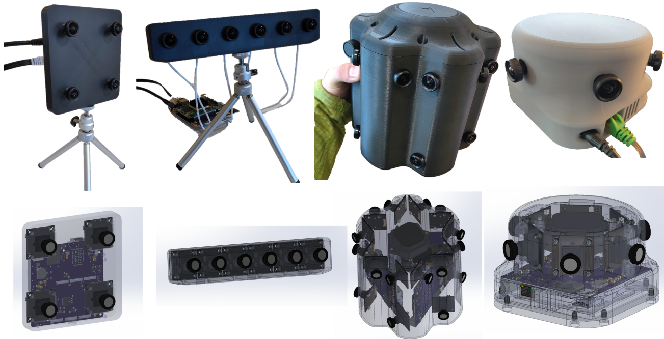
Figure 7: A set of DevCAM multi-camera configurations with their respective CAD designs. From left to right: quadocular, linear light-field, trinocular panoramic and panoramic
