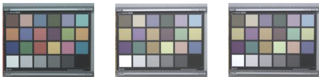
Figure 8. Demosaicking images obtained from (a) RGB, (b) CMY1.0 and (c) CMY2.0 sensors, which are illuminated by D65 under 500 lux.
