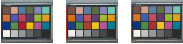
Figure 12. Images reconstructed from (a) RGB, (b) CMY1.0 and (c) CMY2.0 CFA after color correction, which are illuminated by D65 under 30 lux.
