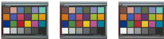
Figure 9. Images reconstructed from (a) RGB, (b) CMY1.0 and (c) CMY2.0 CFA after color correction, which are illuminated by D65 under 500 lux.
