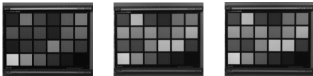
Figure 6. Raw images captured by sensors equipped with (a) RGB, (b) CMY1.0 and (c) CMY2.0 CFA, which are illuminated by D65 under 500 lux.
