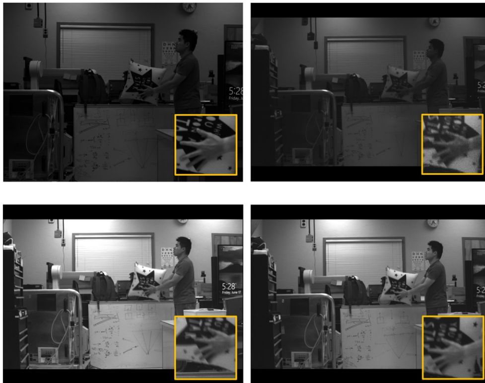
Figure 14. The views of the HFR - LFR array. The exposure time of (a) was 4.3 ms. The exposure times of (b)–(d) were the same, around 12 ms. Since the HFR camera was not synchronized with LFR cameras, (a) was captured \pm 2.15 ms away from the moment that (b)–(d) were captured. The orange windows highlight the moving pillow. The brightness and contrast of the patches in the orange windows were adjusted for display.
