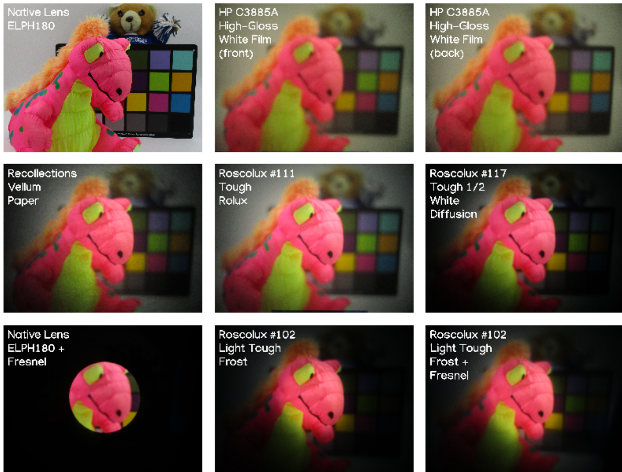
Figure 12. Test scene BSI DCO images using various screens with ELPH180 on CHEM with SMC Takumar 50mm f/1.4
