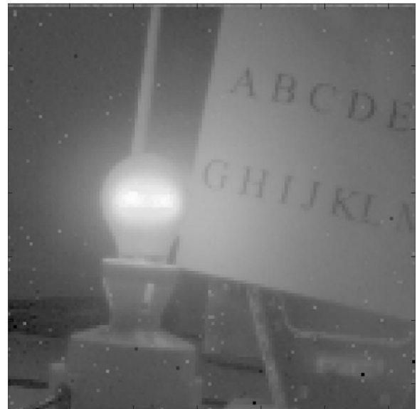
Fig. 5. Image acquired with the proposed sensor. The acquisition time was 14 ms.
